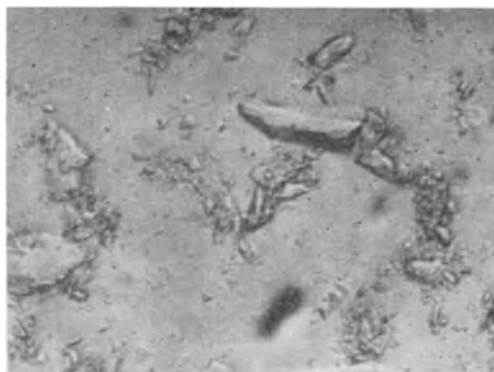
Fig. 2. Photomicrograph of Vycor glass particles. Magnification 1000X.
