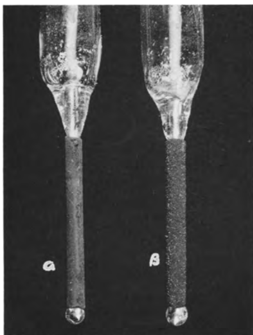
Fig. 1. Electrodes of \alpha - and \beta - \text{PbO}_2 electrodeposited on Pt
