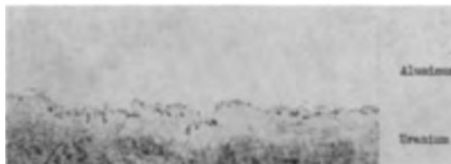
Fig. 6. Aluminum electroplate on uranium after 24-hr diffusion at 200°C (aluminum thickness, 12 mils). As-polished. Magnification 500X before reduction for publication.
