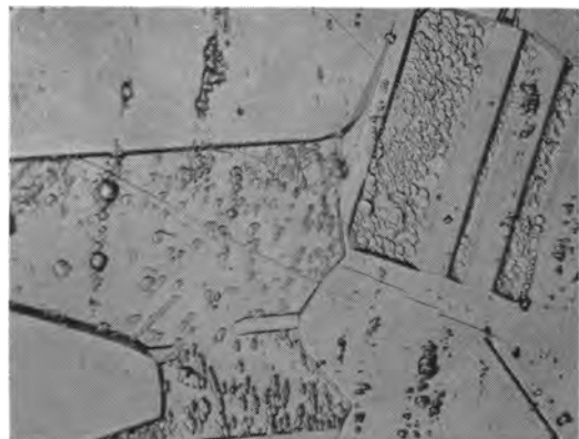
Fig. 13. Electrolytic etch of AISI-316L steel in 10% oxalic acid. Steel: FI-4 (0.020% C, 16.2% Cr) heated 1 hr at 1250°F. Etch: 1 amp/cm 2 for 1.5 min. Step structure: nitric acid corrosion rate 0.04 in./mo. Magnification 500X before reduction for publication.
