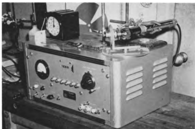
Fig. 2. Apparatus used for scanning the radioactivity on copper single crystal spheres having adsorbed thiourea- S^{36} .
