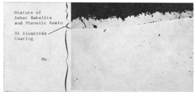
Fig. 3. Ni-aluminide coating. Breakdown after 540-hr exposure to oxidizing flame at approx. 800°C; leaching in 20% HCl; Keller's etch. Magnification 500X before reduction for publication.
