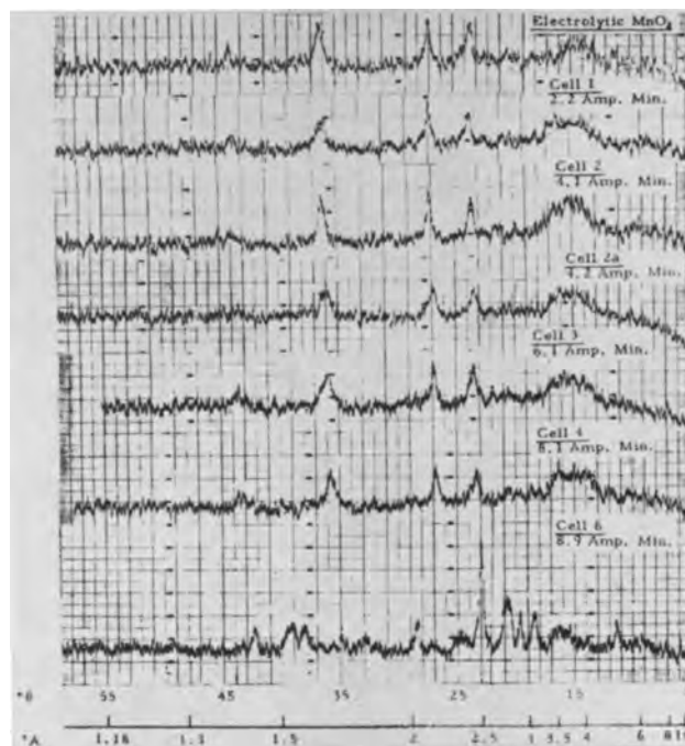
Fig. 5. X-ray diffraction patterns of insoluble cathode products at various levels of discharge.
