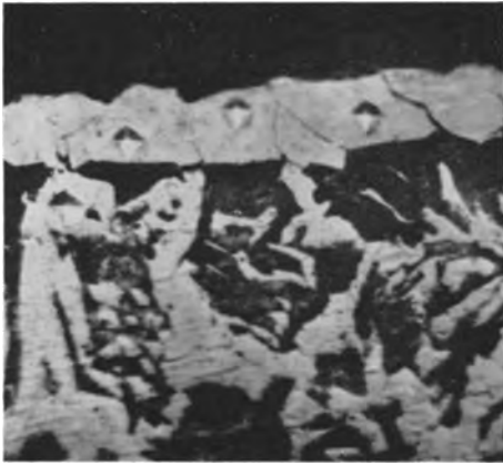
Fig. 5. Micrograph of a section from a sample plated with Ti in a KI-KF bath (Expt. 15, Table I). The microindentations in the Ti deposit correspond to a hardness of about 180 Vickers which is of high order and possibly results from some diffusion of the steel constituents into the Ti coating at the temperature at which the cathode was held during the electrolysis (950°C). 1% HF + Nital etch Magnification: 500X
