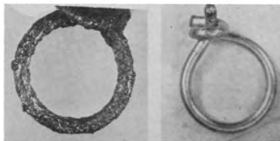
Fig. 2. (a) (left) Rough and nonuniform surface obtained in a KI-NaI bath with TiI_4 addition (Expt. 10, Table I). (b) (right) smooth and uniform coating obtained in KI-KF bath (Expt. 15, Table I). Approx. 2/3 size.
