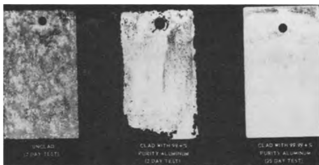
Fig. 1. Bare, 99% Al clad, and 99.99% Al clad AZ31A alloy after exposures to 3% sodium chloride. Period of exposure 7, 2, and 25 days, respectively.
