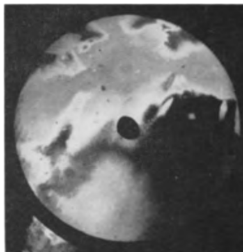
Fig. 7. Copper single crystal oxidized in air-saturated distilled water at 25°C. Lower side was exposed to light from a 3200°K tungsten lamp, upper side kept dark.
