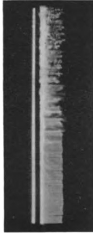
Fig. 1. Transition from laminar to turbulent flow in the electrode film in electrodeposition of Cu under free convection conditions.
