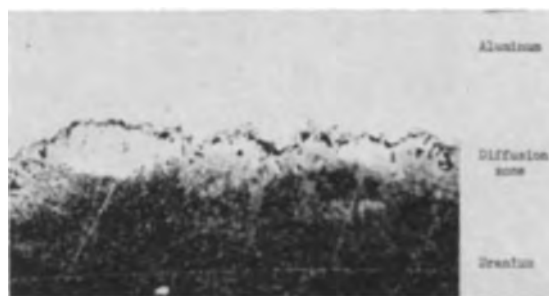
Fig. 7. Aluminum electroplate on uranium after 24-hr diffusion at 250°C (aluminum thickness, 12 mils). As-polished. Magnification 500X before reduction for publication.
