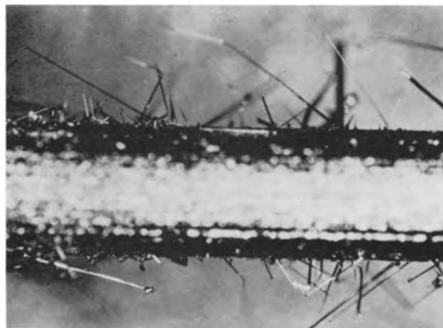
Fig. 6. Iron whiskers from experiment I. Magnification 38X before reduction for publication.
