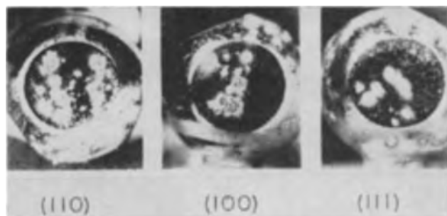
Fig. 1. Three different crystallographic planes of an iron single crystal corroded in distilled water for 3 hr at 25°C. 2.5X.
