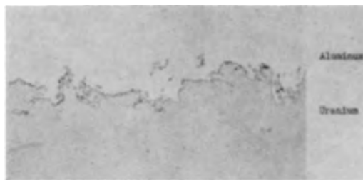
Fig. 5. Aluminum electroplate on uranium as-plated (aluminum thickness, 12 mils). As-polished. Magnification 500X before reduction for publication.
