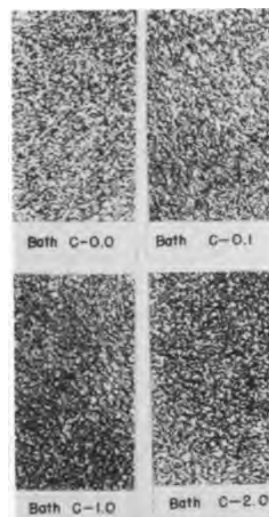
Fig. 15. Effect of magnesium content of Wesley bath on the structure of electrodeposited nickel. Section perpendicular to direction of growth of deposit. Magnification 250X.
