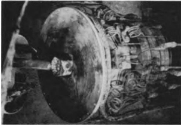
Fig. 2. Anode brush assembly showing anode crater. Graphite cathode can be seen as the smaller diameter electrode.
