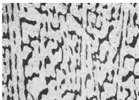
Fig. 12. \text{Cu}_2\text{O} formed on \{110\} plane of Cu by conversion of CuO which was present initially. The change was caused by introduction of \text{CO}_2 into aqueous solution. Magnification 1000X before reduction for publication.
