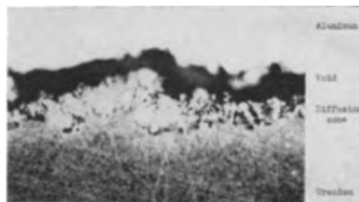
Fig. 8. Aluminum electroplate on uranium after 24-hr diffusion at 300°C (aluminum thickness, 12 mils). As-polished. Magnification 500X before reduction for publication.
