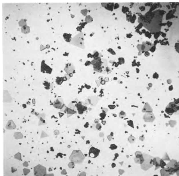
Fig. 4. Display of SiC crystallites as they fell in the furnace. Graphite dust and silicon spheres are also present. One inch equals 40 mils.
