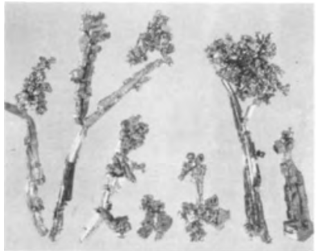
Fig. 2. Titanium crystals 99.8% Ti, BHN 110, made by two-stage electrolysis from TiC. Magnification X8.
