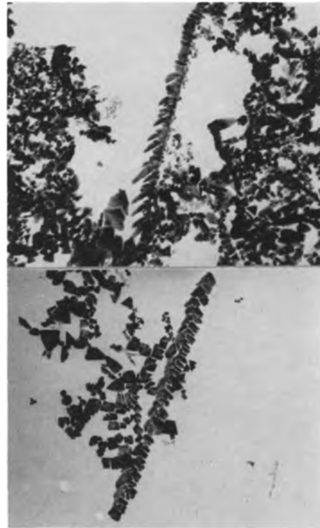
Fig. 30. Electron photomicrographs of carbides isolated from sensitized AISI-316 steel. Steel: GT-8, specimens same as Fig. 29. A (top), from small-grained specimen; B (bottom), from large-grained specimen. Magnification 20,000X before reduction for publication.
