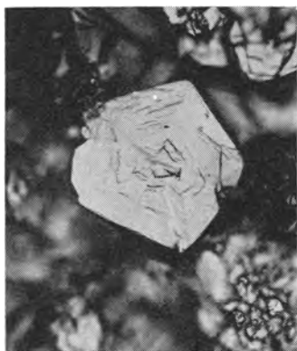
Fig. 4. Surface view of crystalline electrodeposited aluminum. Magnification approx. 1000X before reduction for publication.
