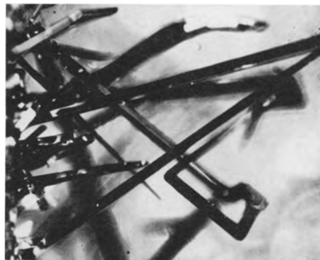
Fig. 7. Iron whiskers from experiment H. Magnification 38X before reduction for publication.
