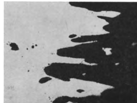
Fig. 4. Type of oxidation fingers formed by oxidation of Mo on breakdown points of Ni-aluminide coating at 800°C. Magnification 500X before reduction for publication.
