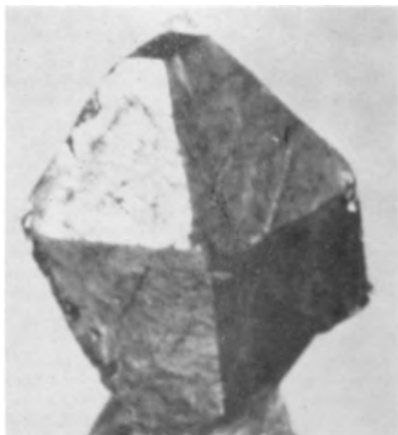
Fig. 3. Single crystal of SiB 6 . Magnification 22X
