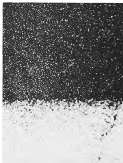
Fig. 8. Boundary between dark and illuminated areas of Cu single crystal surface oxidized in air-saturated distilled water at 25°C. Upper region kept dark, lower illuminated. 500X.
