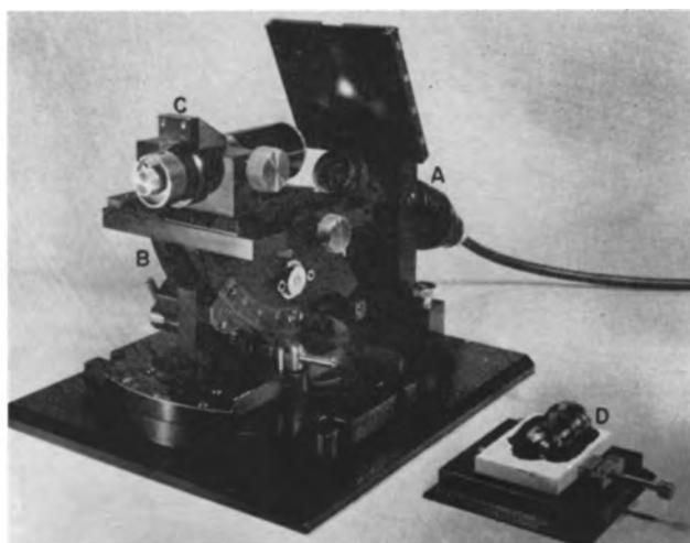
Fig. 2. Instrument for optical orientation: A, optical system; B, goniometer, transferable to cutting machine; C, third circle attachment; D, ingot mounted for orientation and cutting.
